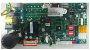
Solution: Check the connecter of indoor motor and slot (CN3) and (CN4), if loose or not plugged in, please connect again.
