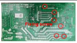
Heat radiation problem easily happened while the screw is not fixed tightly.
