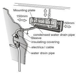
Install the indoor unit at a height of at least 2.5m from the ground.
