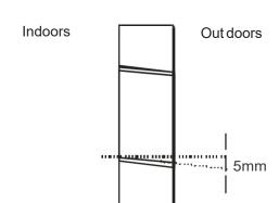
The hole must slope downwards towards the exterior. Note: Keep the drain pipe down towards the direction of the wall hole, otherwise leakage may occur.
