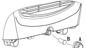
When the water tank is full, "E2" will be displayed on the display Please remove the rubber cap "B" of the drain hole to drain out the first. After the drainage is completed, please restart the unit and then unit can operate normally.
