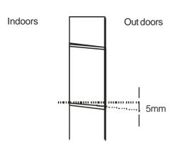
The hole must slope downwards towards the exterior. Note: Keep the drain pipe down towards the direction of the wall hole, otherwise leakage may occur.
