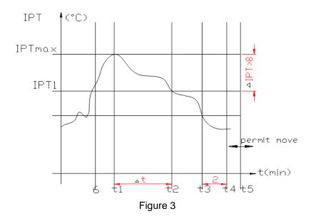
Condition 2: When running time is more than or equal to 120 min (compressor is running accumulatively), the indoor temperature is less than 35°C for 2 min sustained. Running into defrosting under condition 2, defrosting time set is 8 min.
