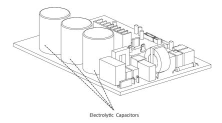
For other models, connect discharge resistance (approx.100 ∧ 40W) or a soldering iron plug between the positive ahegative terminals of the electrolytic capacitor. The terminals are located on the bottom surface of the outdoor PCB.
