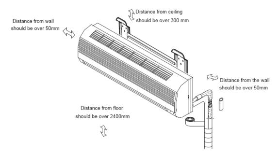
Note: a.The wallboard must be smooth and straight, with its supporting force of not less than 60 kg.
