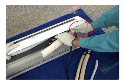
**Note**: When you bend the evaporator pipe, you should use your right hand hold the pipe tightly at bends, and then use the left hand bend the pipe slowly.
