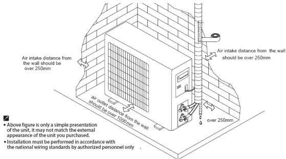
Note: The wallboard supporting force should be able to withstand four times the weight of the outdoor unit, and not less than 180 kg.
