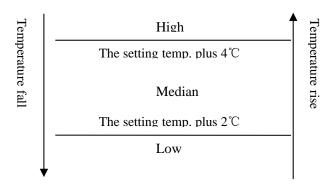
When the difference between the setting temperature and the room temperature equal to  $2^{\circ}$  or  $4^{\circ}$ , the indoor fan speed will keep in current speed.
