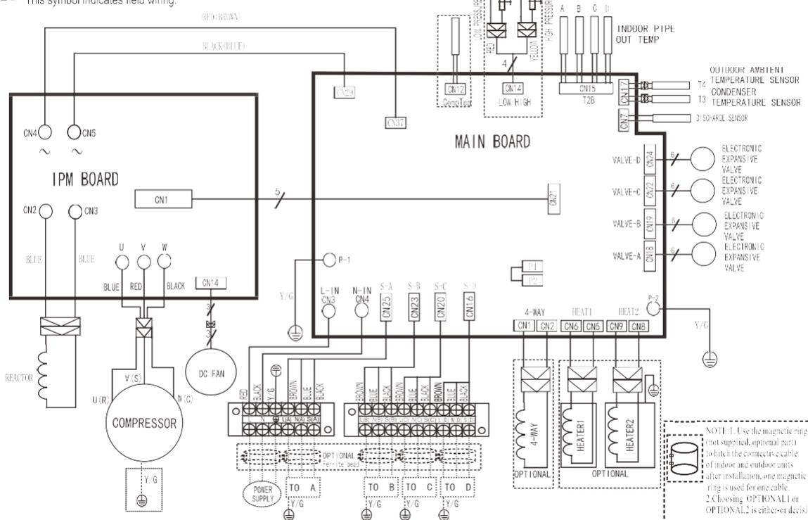
NOTE: 1. Use the magnetic ring (not supplied, optional part) to hitch the connective cable of indoor and outdoor units after installation, one magnetic ring is used for one cable.
