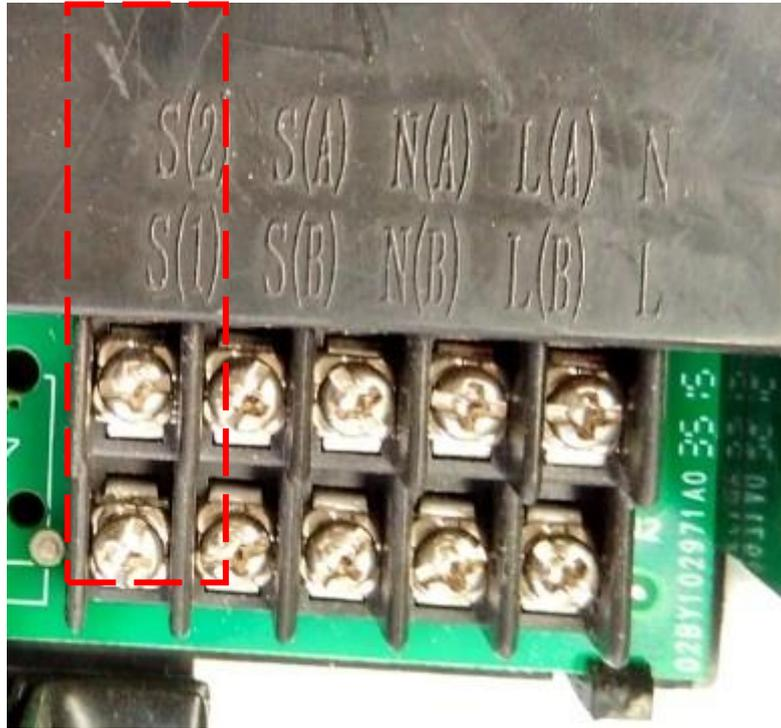
Note: S(1)&S(2) are used in other type of models. They don't need to be connected in multi models.
