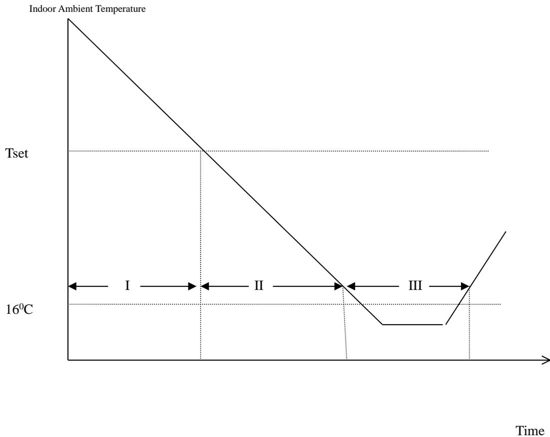
Dehumidifying area I: Operation at the frequency in the range (30–60Hz) according to  $\Delta t$  ( $T_{\text{indoor ambient}} - T_{\text{set}}$ ).
