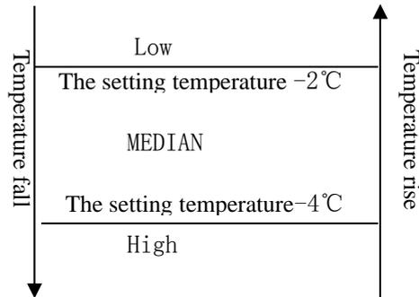
When the difference between the setting temperature and the room temperature equal to  $2^{\circ}\text{C}$  or  $4^{\circ}\text{C}$ , the indoor fan speed will keep in current speed.
