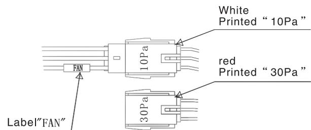
Fig. 7.2 10Pa or 30Pa Static Pressure of Change
