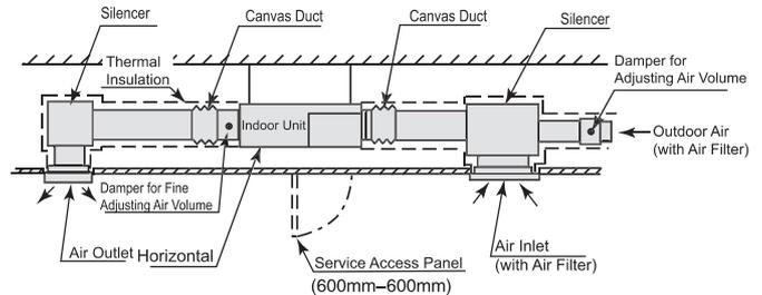
Fig. 4.8 Duct Connection
