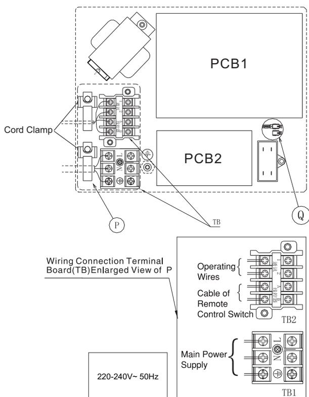
Fig 7.3 Electrical Wiring Connection
