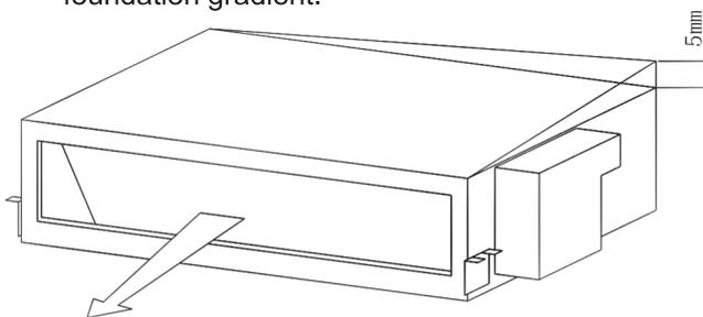
Fig. 4.7 Foundation Gradient
