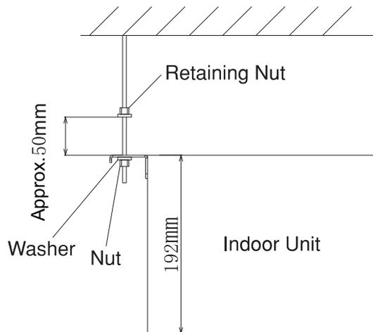
Fig. 4.5 Sling Bolts and Nut
