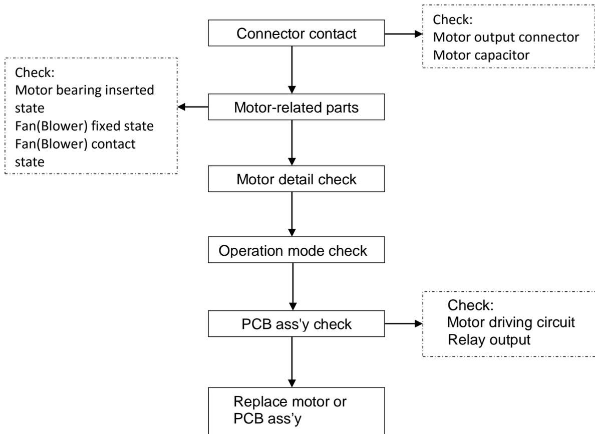
**10.3 Compressor or outdoor fan does not operate at all.**
