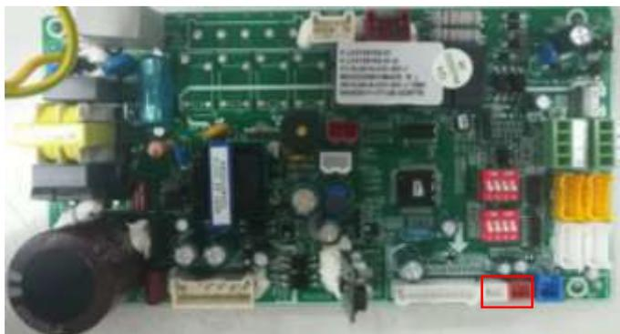
**Solution:** Check the connector of sensor and slot (CN6, CN6-1, CN6-2), if loose or not plugged in, please connect again.
