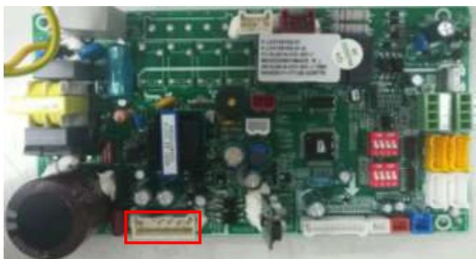
**Solution:** Check the connector of indoor motor and slot (CN3) and (CN4), if loose or not plugged in, please connect again.
