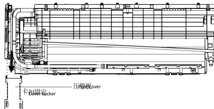
9. Disassembly the evaporator
