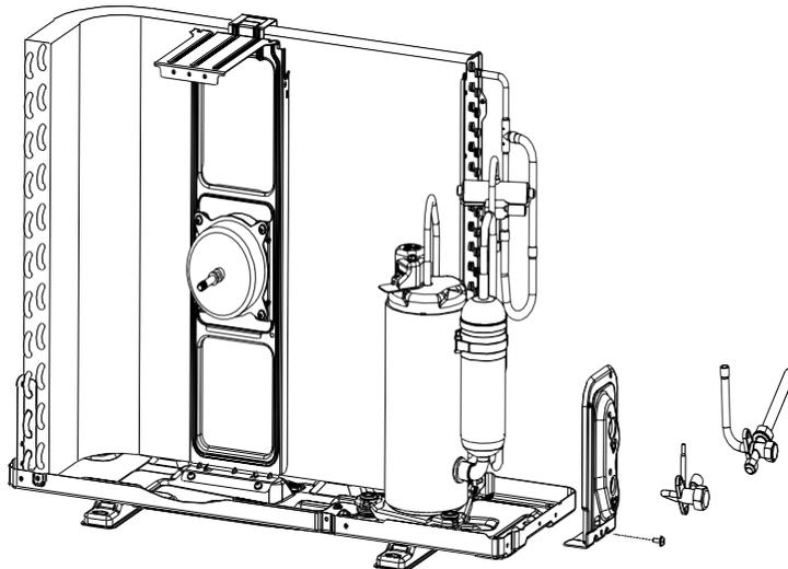
**step9: Disassemble the 4-way valve assembly**
