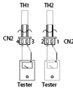
**TH1: indoor room temperature sensor and outside air temperature sensor**
