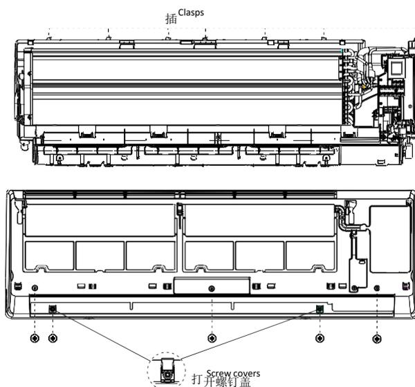
7. Disassembly the electric control box.
