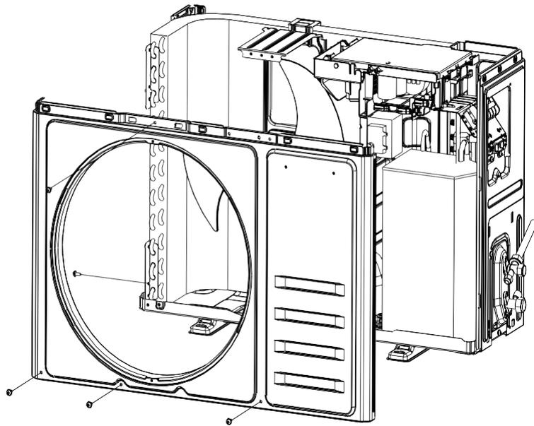
**step3: Disassemble the Left and Right plate.**
