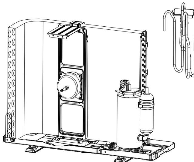
**step10: Disassemble the compressor.**
