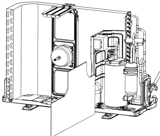
**step7: Disassemble the separate plate**
