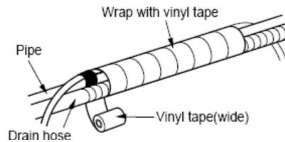
**2.5.6 Indoor unit condensed water drainage**
