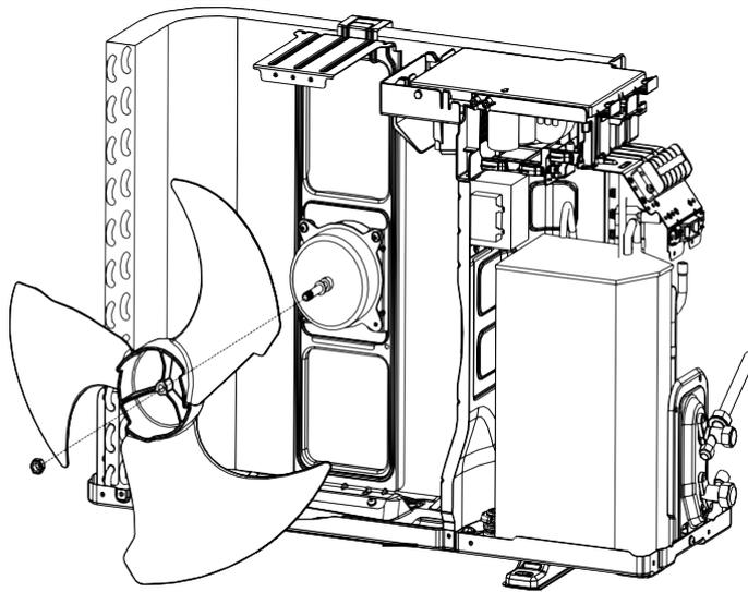
**step5: Disassemble the electric box**
