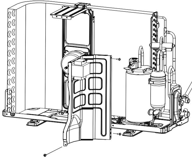
**step8: Disassemble the 2 and 3-way valve**
