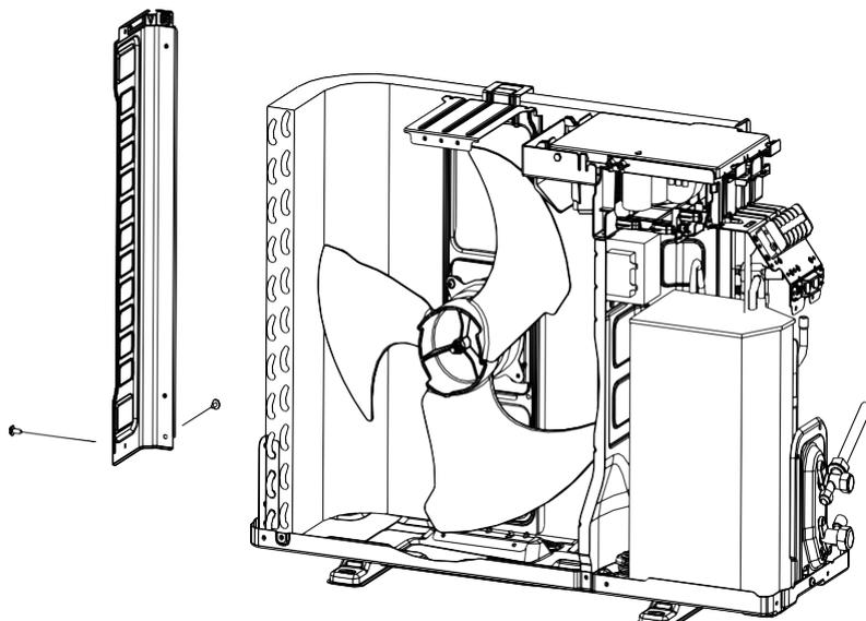
**step4: Disassemble the Axis Fan Blade**
